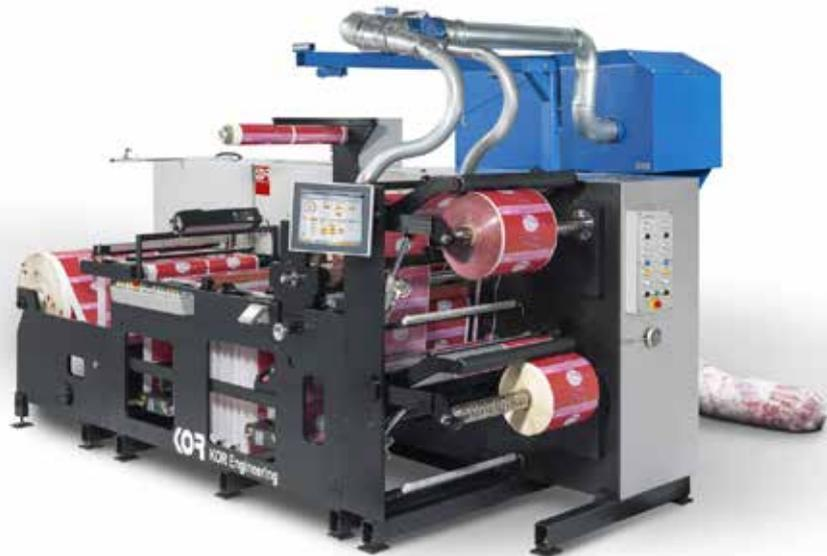
*that handles up to heavier 40" rolls. It also boasts precise tension control and high-speed defect placement, so a single operator can inspect, edit, slit and rewind in one efficient step. Another notable feature is the ability to integrate a vision system and a 2-in-1 shear/razor slitter.*
